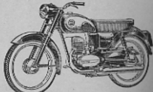
MODEL K7 — CAPTAIN 200 First frame number BK7/1928 Villiers 197 cc. Mk. 10E engine
