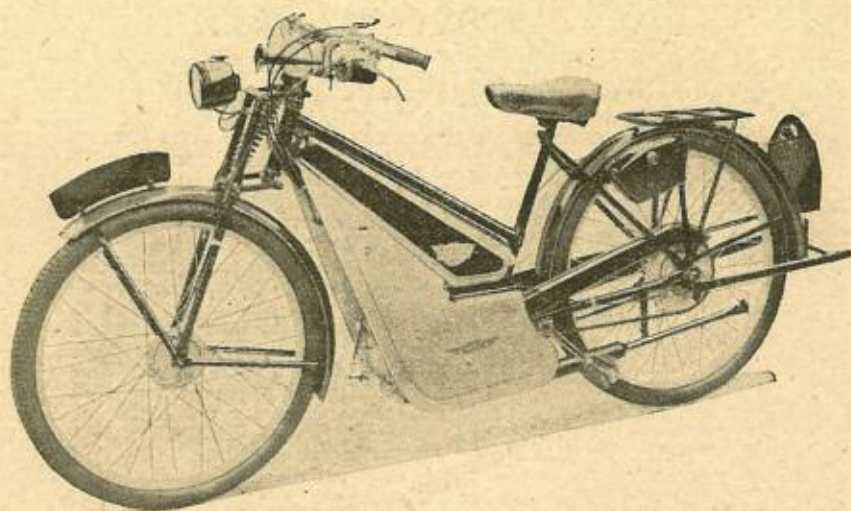
With its shielding, Argenized finish and single-tube telescopic-looking spring forks, the James "Superlux" autocycle has a most attractive appearance
