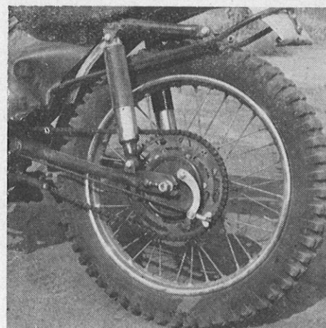
Rear view of the modified James quickly shows some desirable features: ultra light rear sprocket and tent around carburetor (not standard equipment); sturdy swing-arm suspension and sports tire.
